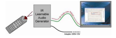
You are ready to record the IR-code. Make sure that both the audio remote control and the TELETASK RS232/learnable interface are close at hand.
