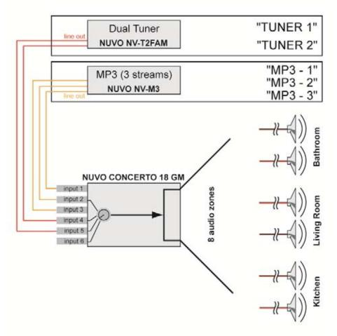
The schematic structure of the audio configuration.
