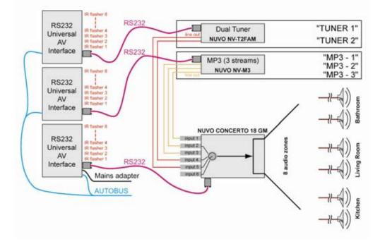
With the assigning of the RS232 Port and assigning names to the sources, the schematic drawing is now finalised. In the next phase, this schematic is used to integrate the whole installation in to the TELETASK 'AV-SOFT' software.
