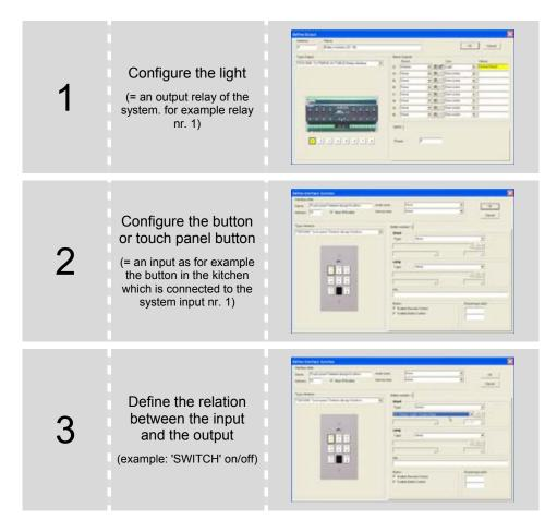
Another very powerful relation can be the control of a number of outputs (loads) by only one button. This seems more complex, but you can define the relation between the button and the different outputs in only three steps.
