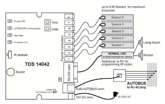
Because the learnable RS232 UNIVERSAL AV INTERFACE is a set top box, TELETASK has chosen for a more aesthetical connection to the AUTOBUS. This connection runs over a short CAT5 patch cable to a RJ45 plug in the wall. Behind the wall plug the AUTOBUS is available. In the table below you can see how the pinning of the CAT5 cable corresponds with the AUTOBUS wires.
