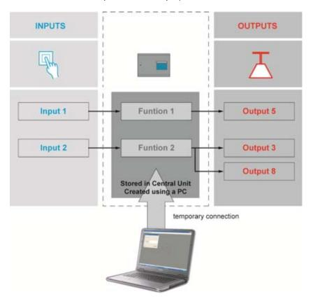
The relations can be defined by yourself, by means of PROSOFT software. PROSOFT was specially developed by TELETASK to make it possible that you can define all inputs, outputs and the relations between them on a standard MS Windows based PC. As soon as your relations are defined, they can be downloaded to the TELETASK central unit which will keep them in his non volatile memory, where they always remain after disconnecting the PC, even when power fails for short or long (unlimited) periods.
