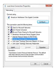
Now you will get a window where you can set the IP configuration for your computer. Change the settings so it looks like this (Assuming that the IP address of the Micros is 192.168.0.200. If not, make sure that the 3 first numbers are the same as from the IP address of the DOIP and that the last number is different). Warning: Note the settings. Before changing them you might need them in order to reconnect your computer to a network or Internet afterwards.
