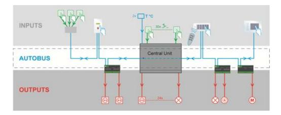
With this way of working there is still something missing because there is nothing which defines yet that the push button on the wall is for example going to control the ceiling light in the dining room. Therefore the system needs a relation which is to be defined between that particular input and the related output.
