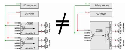
Today there are several power amplifiers with built-in audio sources. In small tower systems you have all common sources built-in, but even some higher range power amplifiers may have a built in radio tuner or hard disk. The most important and typical feature of such systems, is that the built-in sources are not to be shared with other power amplifiers. You can find a comparing illustration in figure 5.
